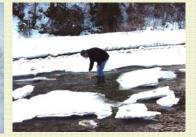
The tracer is injected a good distance upstream (here: 10 g naphtionate diluted in 1 liter). The success of the method relies on the perfect mixing on a cross-section of the stream at the measurement point.
