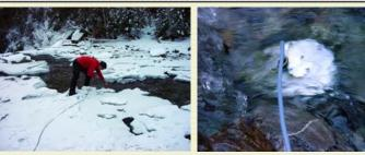
2nd step : Installation in the stream Without stopping the data acquisition, the fluorometer is installed in the stream. The background signal is recorded during a few minutes. Note that this background signal can be particularly high at the excitation wavelength used for naphtionate, due to the presence of DOC. For uranine or rhodamine, this level is below 1 ppb. Since the background is subtracted from the tracer signal, the only requirement is that the background signal remains stable.
