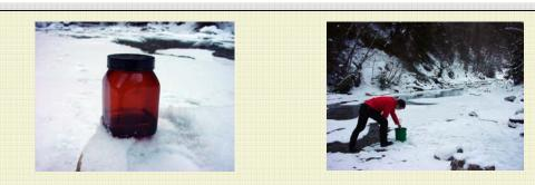
1st step : Local calibration of the fluorometer with steam water A ready-to-use volume (50 ml) of a solution of tracer at 10'000 ppb is mixed with water from the stream to make 5 liters of calibrating solution at 100 ppb concentration. The fluorometer is immersed in this solution, switched on and set for 2second sampling rate. It is kept running all the time till the end of the measurement. This allows for the display of the calibration and breakthrough curves on the same screen.
