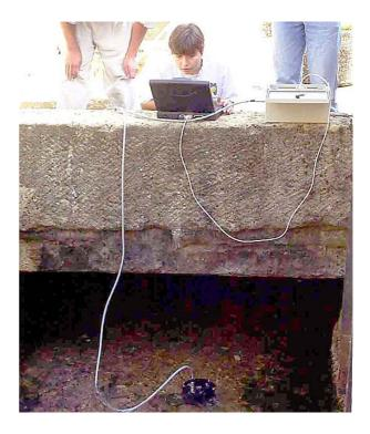
Figure 3 - Field fluorometer set-up in a stream
