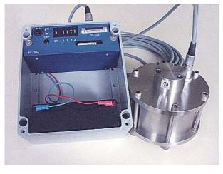
Figure 1 - Flow -through field fluorometer probe with datalogger. As many as four optics allow detection of any dye tracer with excitation band between 370 and 600 nm.
