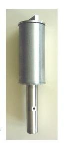
Autonomous suspended fluorometer for tracer tests in submarine aquifers
