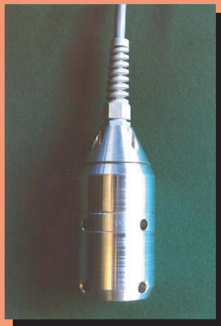
Fig. 2: Downhole fluorometer FL10, showing lateral inlet/outlet holes. Sonde diameter: 74 mm Height: 200 mm
