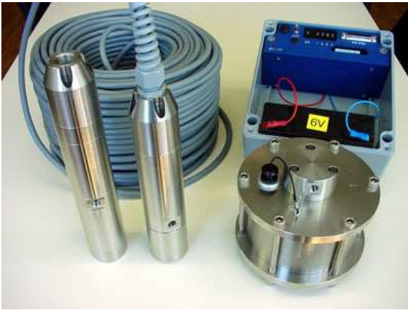
Fig. 2: Field fluorometers (L: 2" downhole, R: surface waters) and a data logger with flash card and battery.
