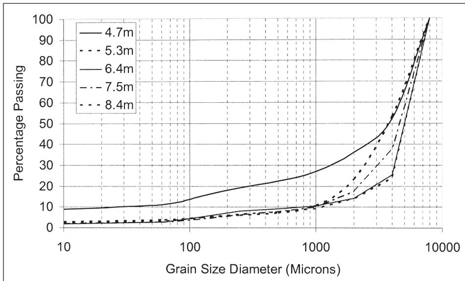
Fig. 2: Representative grain size distribution analyses for samples of aquifer material collected from depth corresponding to the screened interval of K3-2, Kappelen, Switzerland. Hydraulic conductivity estimated from Hazen rule (R. A. FREEZE & J. A. CHERRY, 1979).
