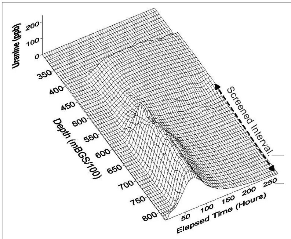
Fig. 5: Composite depth-specific breakthrough curve generated using mobile downhole fluorometer, K3-2, Kappelen, Switzerland. Note: Tracer storage above screened interval due to tracer displacement by fluorometer during successive measurement cycles.
