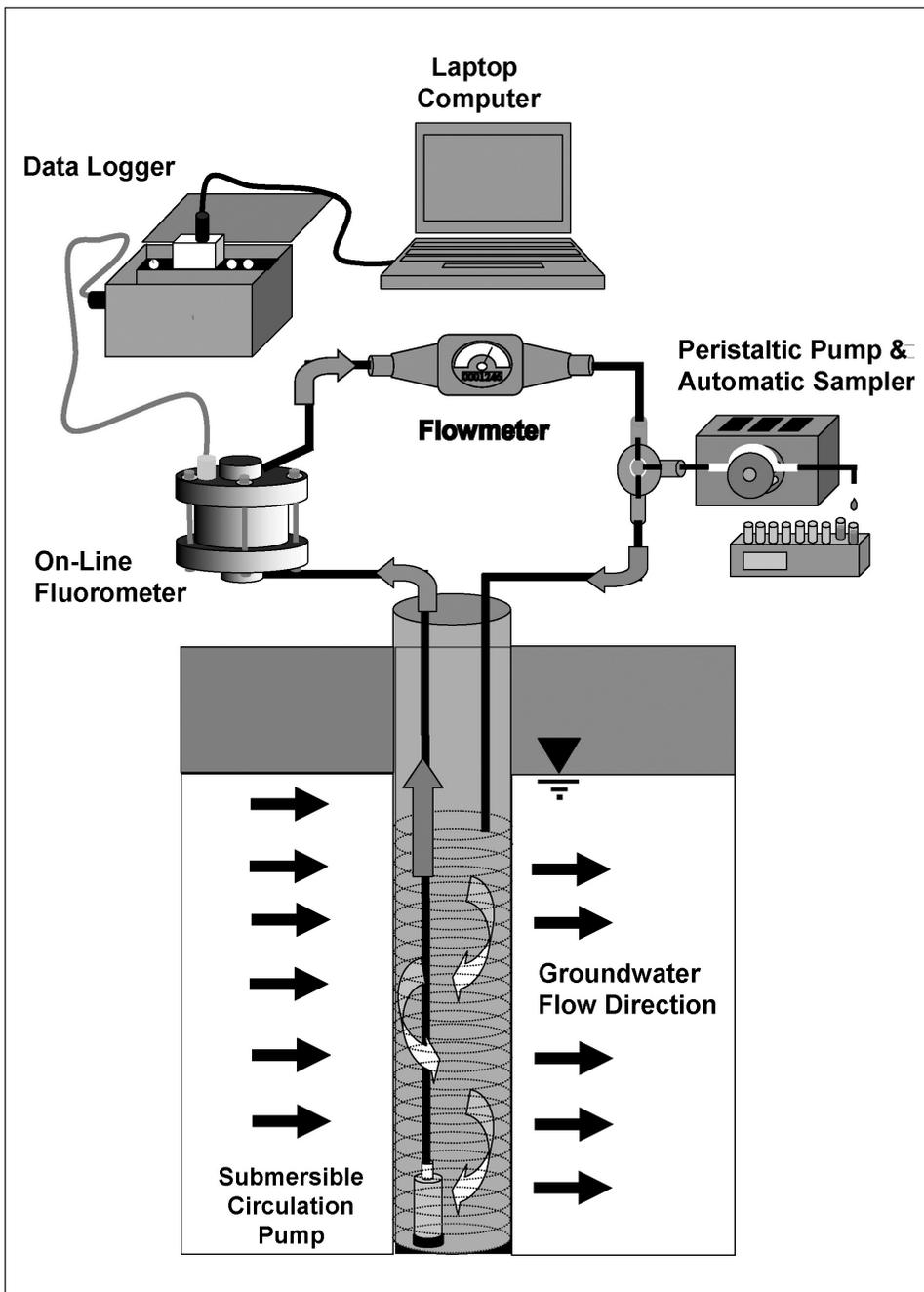
Fig. 3: Continuous circulation apparatus used to monitor tracer concentrations in injection well, K1-2 and observation well, K3-2. Note: Automatic sampler not used in injection well setup.
