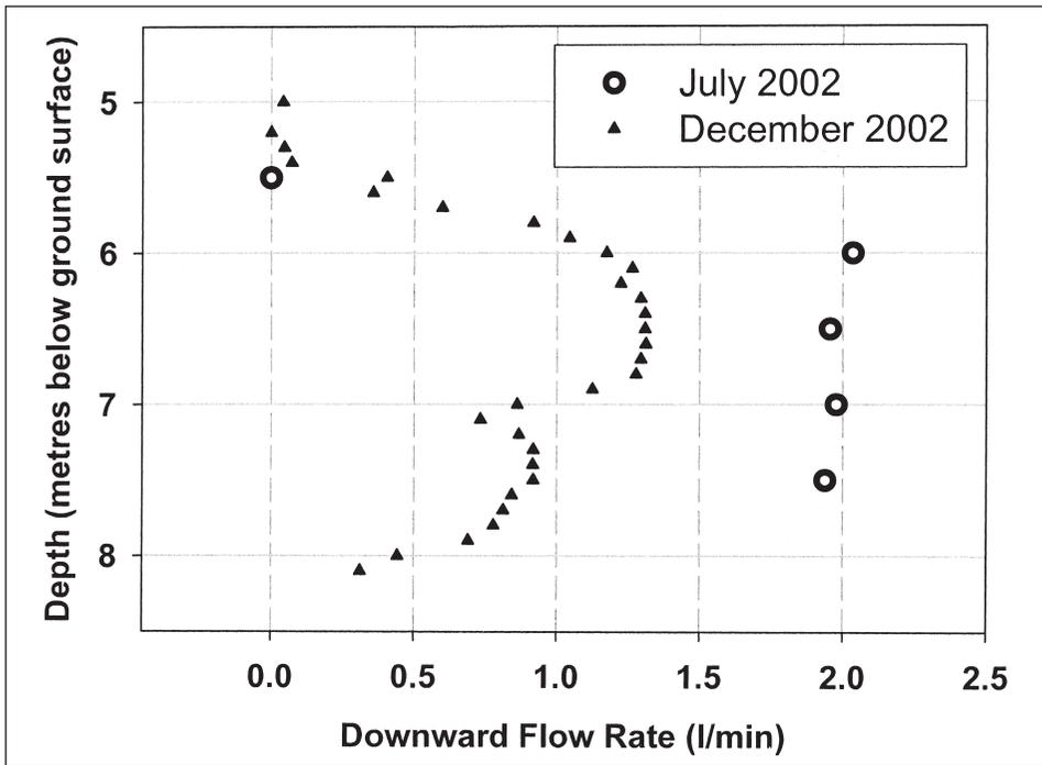
Fig. 6: Downward flow rates in K3-2, Kappelen, Switzerland, measured using heat pulse flow meter in July 2002 and December 2002.
