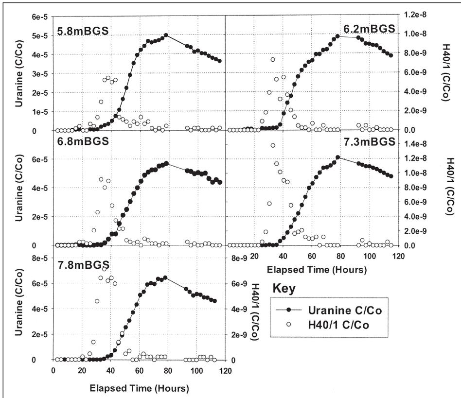
Fig. 4: Breakthrough curves for five different depths sampled using a multichannel low-flow sampling system at K3-2, Kappelen Test Site, Switzerland.  $C/C_0$  – injectate concentration, m BGS-metres below ground surface.
