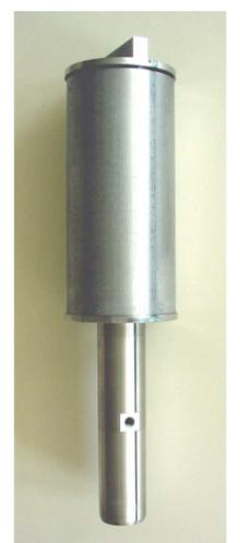
Autonomous suspended fluorometer for tracer tests in submarine aquifers
