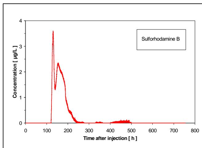
Fig. 3. Tracer test at Lake of Lessy during high water.
