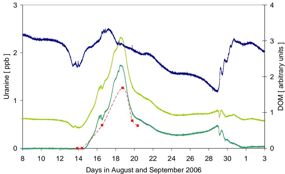
Fig. 2. DOM signal removal from the uranine curve. From top to bottom: DOM curve, uncorrected uranine, corrected uranine, broken line: laboratory analysis of tracer for comparison
