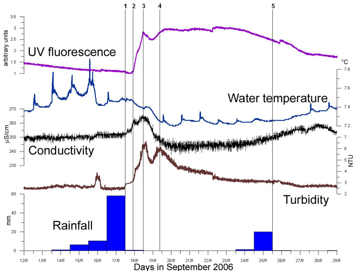
Fig 6. Series of typical events marked 1 to 5 during rise in the water level after rainfall. Daily spikes in water temperature is caused by poor isolation from the air. UV fluorescence results from dissolved organic matter (DOM). Rain height was recorded in the nearby valley of Grand Bornand
