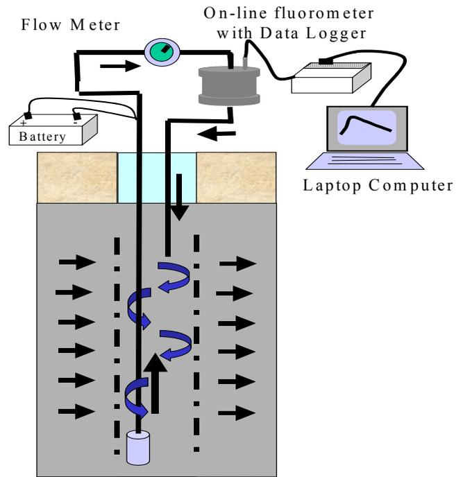
**Figure 7:** Schematic illustration of continuous circulation technique. Water is pumped from the base of the well across the flow-through fluorometer cell before being re-injected. Consequently no net drawdown results.
