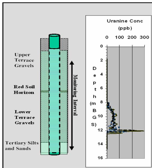
**Figure 10:** Maximum Tracer Concentrations Observed in Well B8, Dornach Using a Mobile Downhole Fluorometer.
