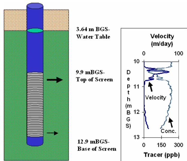
**Figure 9:** Example of identification of zones of preferential groundwater flow using a downhole fluorometer.
