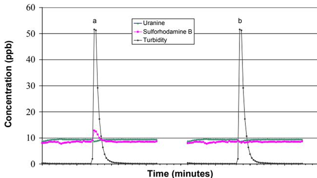
**Figure 4:** Influence of turbidity on tracer concentration measurement, without (a) and with (b) correction.
