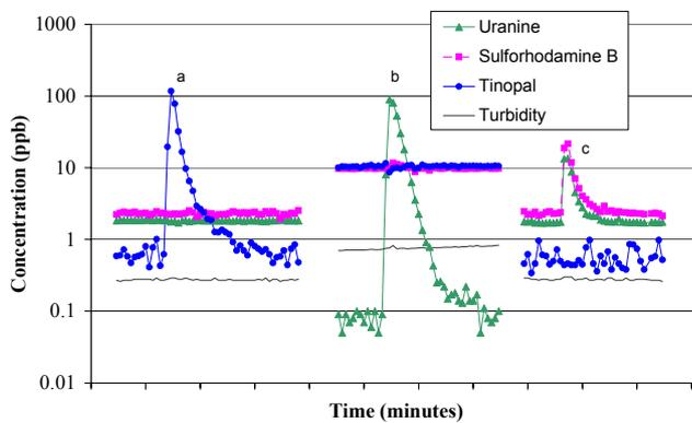
**Figure d:** a,b: Dynamic behaviour of the separation scheme. c: Erroneous signal produced by uncalibrated tracer (eosine).
