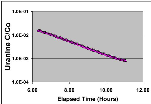
**Figure 8:** Plot of Relative Uranine Concentration with Time for K1-1 Injection Well, Kappelen Test Site. July 2001. Sampling Frequency: Every 4 minutes.
