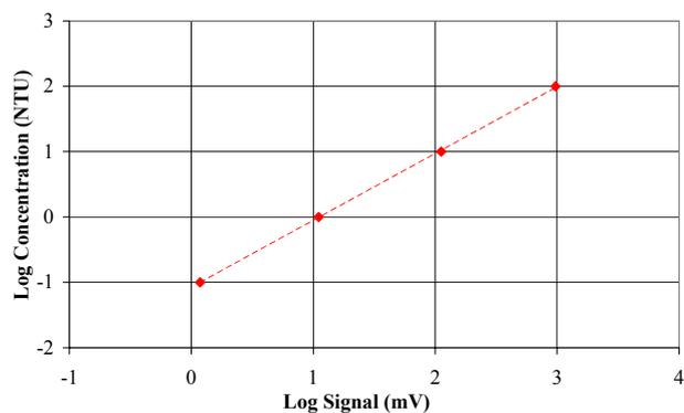
**Figure 3:** Calibration curves for turbidity
