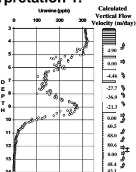
Figure 8: Single well dilution test profile of Uranin concentration in B8 collected measured using mobile downhole fluorometer. Arrows and figures on left hand side of plot are directions and magnitudes (m/day) of vertical flow. (Horiz=horizontal flow). Note tracer arrives at approx. 12mBGS but then flows upward to 9mBGS where it re-enters the aquifer.
