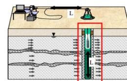
Figure 4: Operation of downhole fluorometer. Pulley draws fluorometer over interval L at ground-surface corresponding to equivalent depth interval in well.
