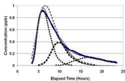
Figure 5: Representative Uranin breakthrough curve observed at B8. Field data in blue; best fit single advection-dispersion term in grey; partial breakthrough curve (dotted) and composite curve (solid) in black.
