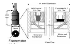
Figure 3: Construction details of downhole fluorometer
