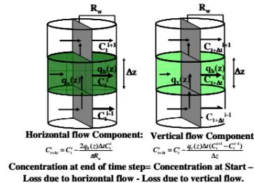
Figure 9: Schematic illustration of mass balance modelling process. Decline in tracer concentration in a cell of thickness  $\Delta z$  during a time step  $\Delta t$  results from removal by vertical flow across the cell  $q_v(z)$  and by Horizontal Flow  $q_h(h)$  into the aquifer.
