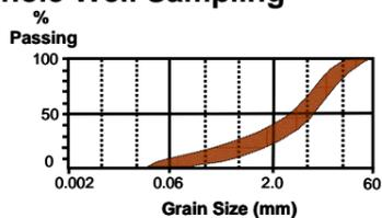
Figure 2. Range of grain size distribution curves for Dornach Aquifer samples. (After Seiler, 1975)
