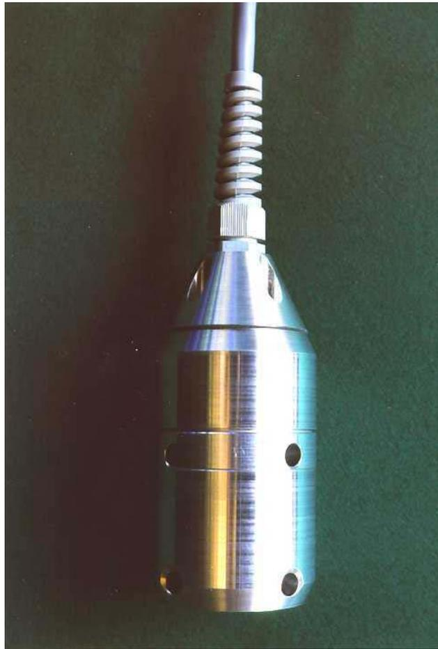
**Figure 1.** Borehole fluorometer probe
