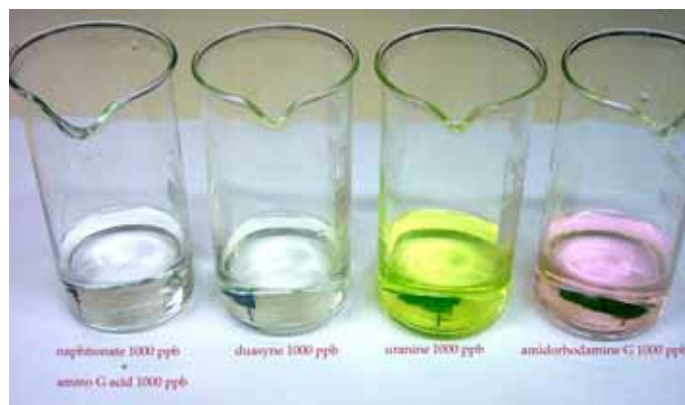
Figure 1 Visible impact of usual dye tracers (concentration: 1000 ppb). The impact is very high for uranine (green) and amidorhodamine G (red), but very weak for duasyne and nil for naphthionate and amino G acid.
